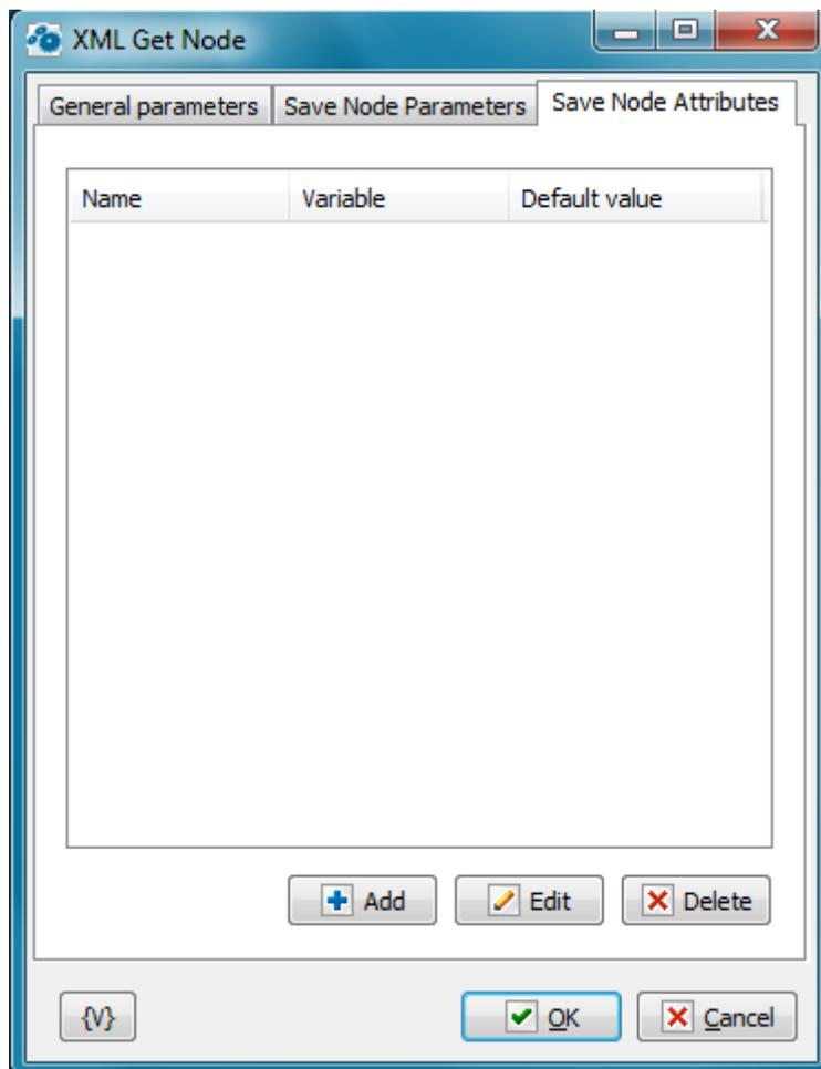
On this tab one can specify the attributes which values are necessary to be saved into variables. It is necessary to specify parameters for every attribute:
